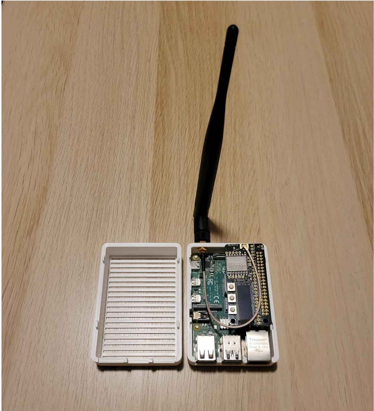
Listing 3: Picture of one of the nodes opened to showcase the internals.
